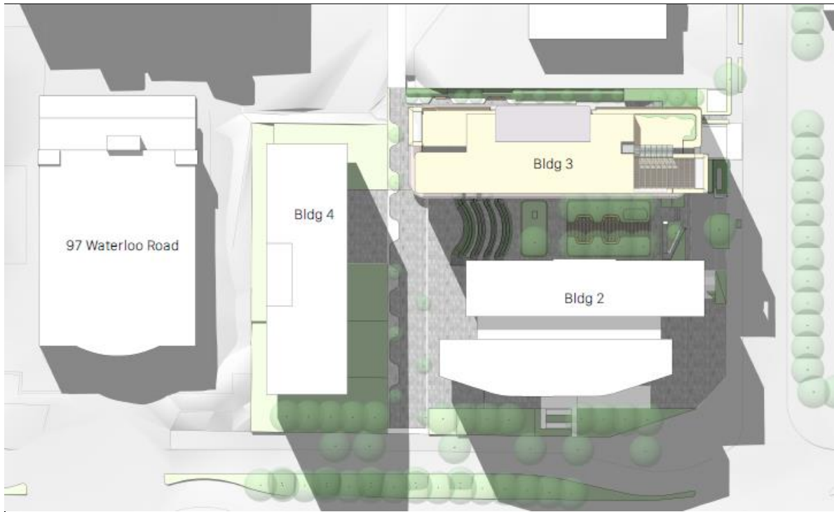
Figure 35: An extract from solar access diagrams. Autumnal Equinox (12:30pm)
